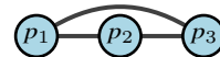
(c) A generically bearing rigid graph in a non-generic position leads to a not bearing rigid framework.
