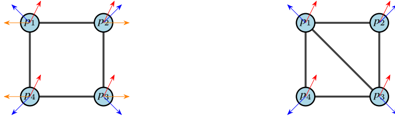
(a) A not infinitesimally bearing rigid frame- (b) An infinitesimally bearing rigid frame- work. work.
