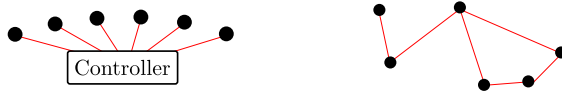
Figure 1.1: Centralized controller that sends corresponding signals to each agents (left). Decentralized controller where each agents calculates its own input signal (right).
