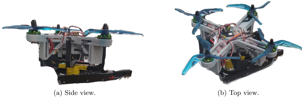
Figure 3.11: Quadcopter mounted in the variable degree of freedom gimbal.
