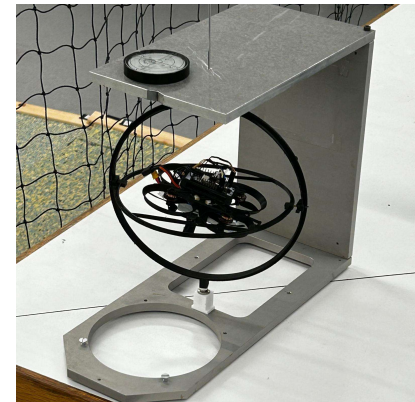
Drone with test stand prototype
